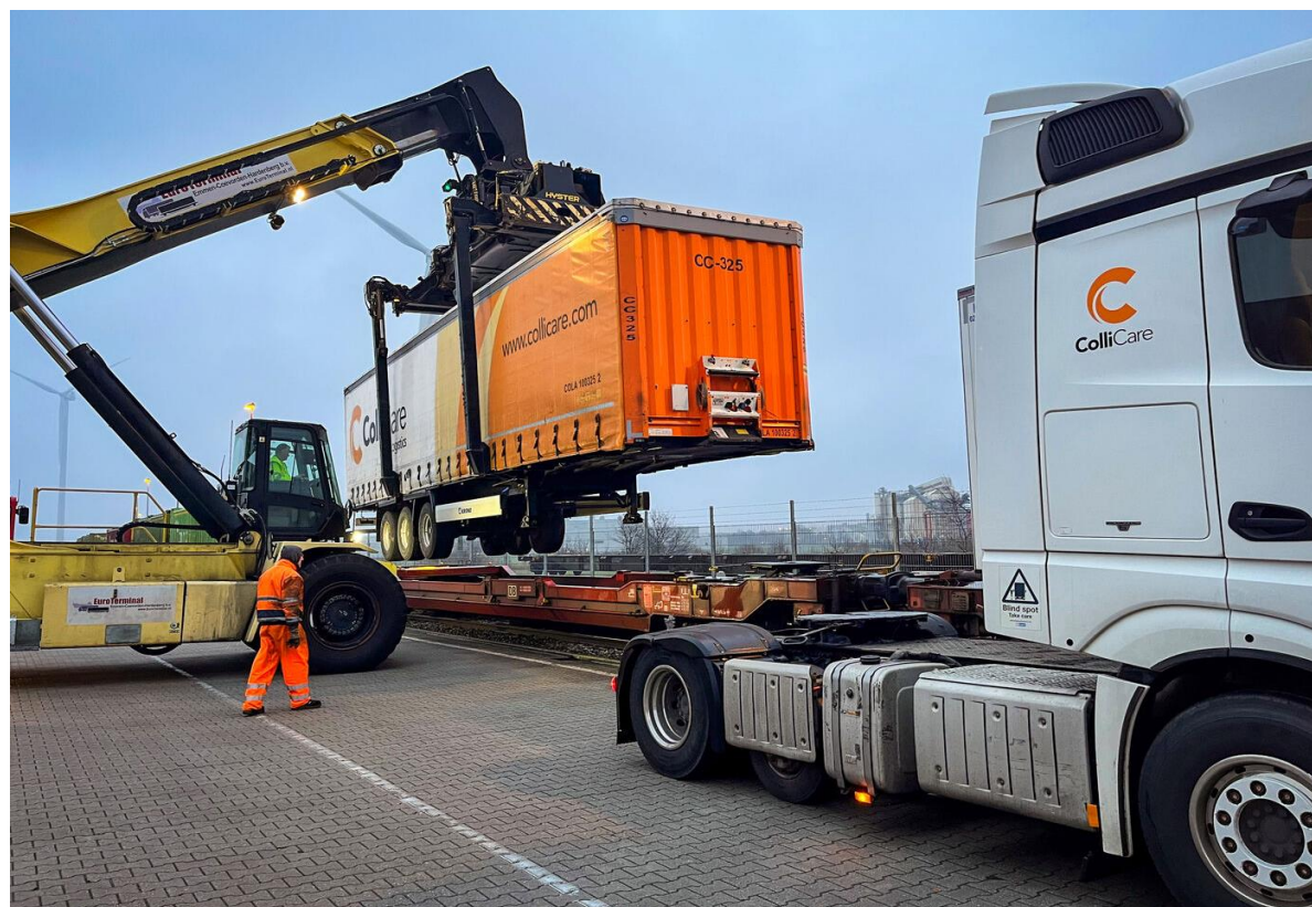
Trailer-on-train transshipment: ColliCare semi-trailer being lifted onto a rail wagon for the cross-European corridor
